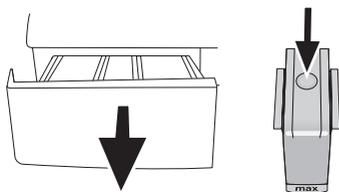
1. Press the dotted point on the siphon in the softener compartment and pull towards you until the compartment is removed from the machine.
