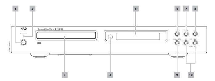
1 **POWER:** Press this button to switch ON the C 515BEE. The Standby LED indicator will turn from amber to blue and illuminate the Vacuum Fluorescent Display (VFD). Pressing the power button again turns the unit back to standby mode.
