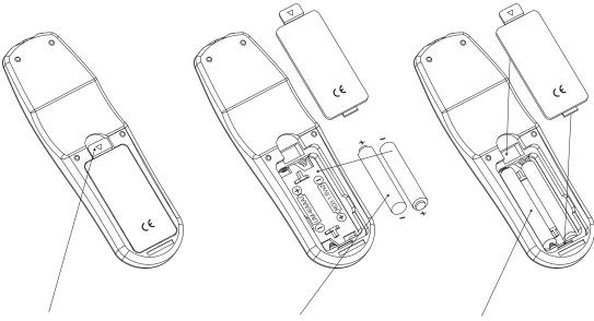
Press batteries into opening. Ensure correct
