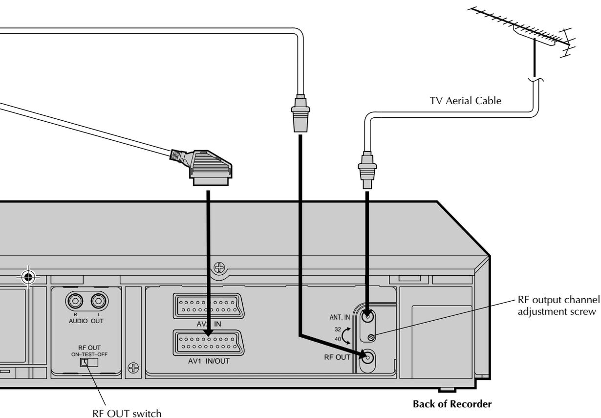
The video recorder sends picture and sound signals via the RF connecting cable to your TV on UHF channel 36.
