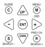
**MENU/OSD button:** Press to display the SYSTEM STATUS screen. From the SYSTEM STATUS screen, press the ENTER button to display the MAIN MENU screen which has links to all other menus. If a menu is already visible, push this button to cancel the display. The MENU button on the front panel provides the same function.
