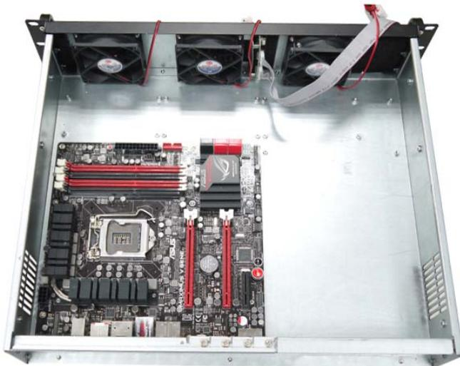
3. Now, you can place a Micro-ATX Motherboard into the chassis, and fasten the screws.
