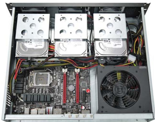
8. For the HDD Cage on the right side, it can take up to 2x 3.5" HDD or 1x 3.5" HDD + 1x 2.5" HDD. You can place the Cage vertically when you are using a standard ATX PS2 power supply (140x150x86mm)
