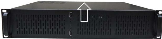
2. Once the screws removed, push the top cover to remove from the chassis.
