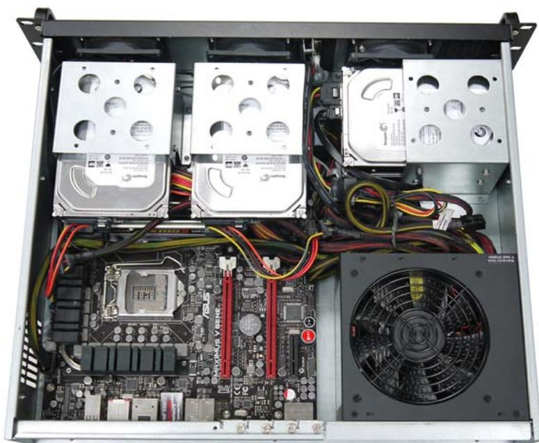
9. You can also place the HDD Cage horizontally if you uses longer ATX power supply (165x150x86mm)
