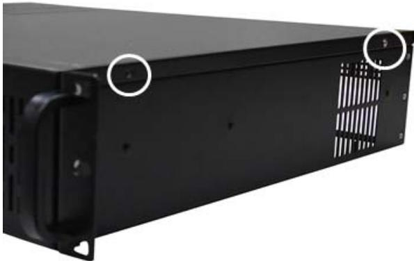
1. Remove the screws from each side of the Chassis. (two on each side)
