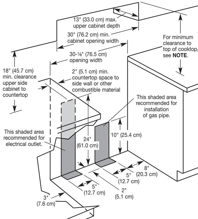
**NOTE:** 24" (61 cm) minimum when bottom of wood or metal cabinet is protected by not less than 1/4" (0.64 cm) flame retardant millboard covered with not less than No. 28 MSG sheet steel, 0.015" (0.4 mm) stainless steel, 0.024" (0.6 mm) aluminum or 0.020" (0.5 mm) copper. 30" (76.2 cm) minimum clearance between the top of the cooking platform and the bottom of an unprotected wood or metal cabinet.
