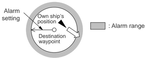
Figure 7-4 How the anchor watch alarm works
