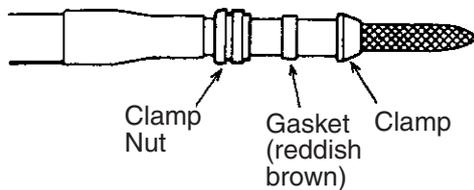
Slip on clamp nut, gasket and clamp as shown left.
