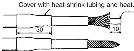
Cut off insulator and core by 10mm.
