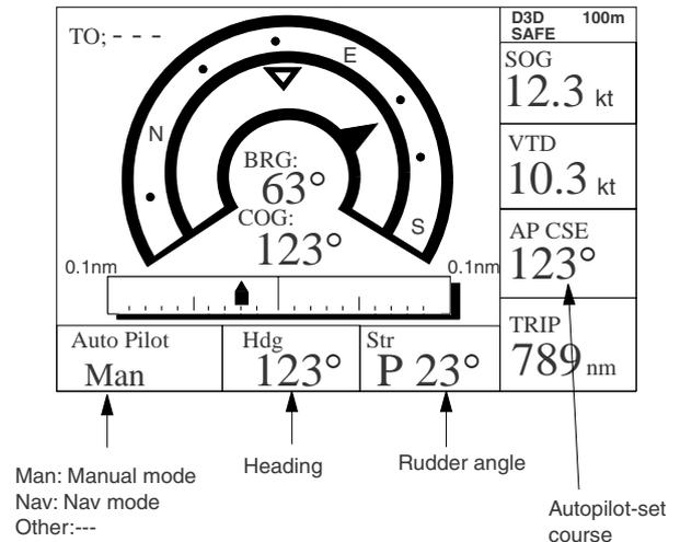
Figure 1-10 Navigation display, autopilot connected, modes other than the automatic mode
