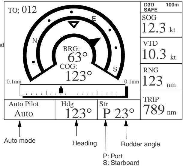
Figure 1-9 Navigation display, with autopilot connected, automatic mode
