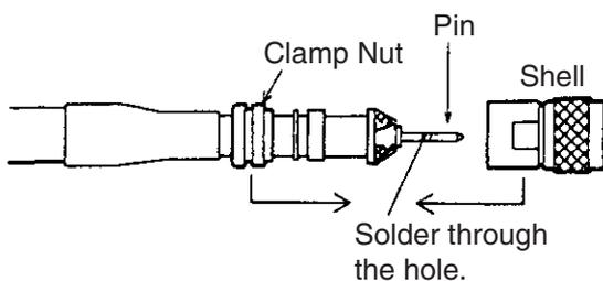
Slip the pin onto the conductor. Solder them together through the hole on the pin.
