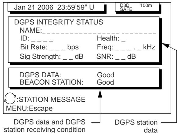
DGPS data and DGPS station receiving condition      DGPS station data
