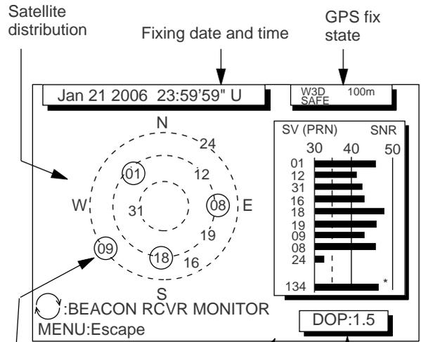
Satellite number with circle is used for positioning.
