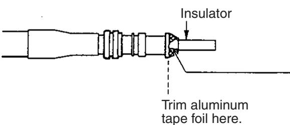
Fold back aluminum foil onto shield and trim.
