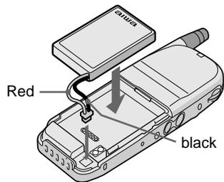
Orient the connector as shown.
