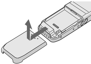
② Connect the battery pack's connector and the PT-H99's connector.
