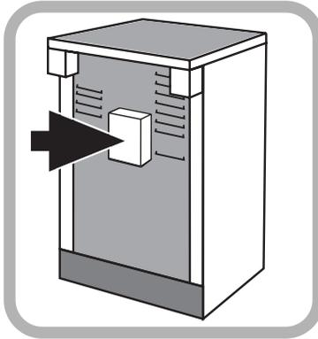
The power supply cable should conform to B.S.6004 with a conductor size of 6mm<sup>2</sup> minimum.
