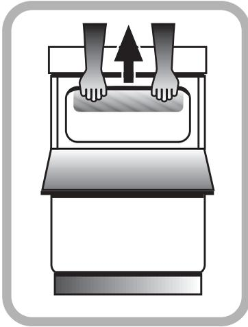
Before moving your cooker check that it is cool, and switch off at the cooker control unit.
