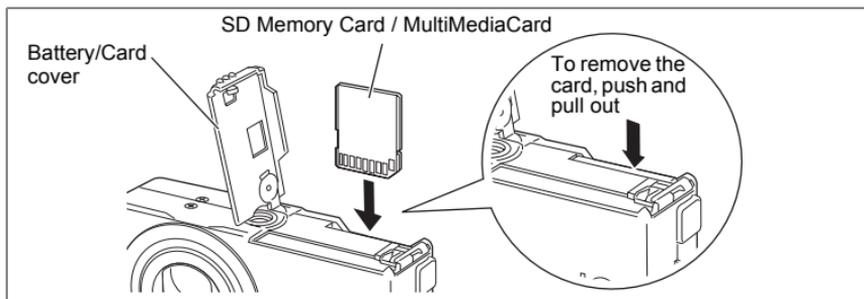
This camera uses an SD Memory Card and MultiMediaCard. Captured images are recorded on the SD Memory Card / MultiMediaCard if a card is inserted (☐ icon on the LCD monitor), or in the Built-in memory if no card is inserted (📷 icon on the LCD monitor). Make sure that the camera is turned off before inserting or removing the SD Memory Card / MultiMediaCard.
