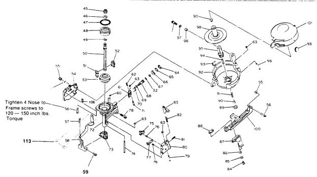
Use Loctite #271 or equivalent when assembling these two screws. Loctite #271 Packet is available as Part No. 851325.
