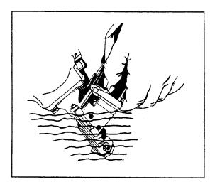
NOTE: Solvents sprayed on nose to clean and free up the trip may have the opposite effect! The solvent may soften the tar on the shingles and cause tar buildup to be accelerated. Dry operation is better, as noted above.
