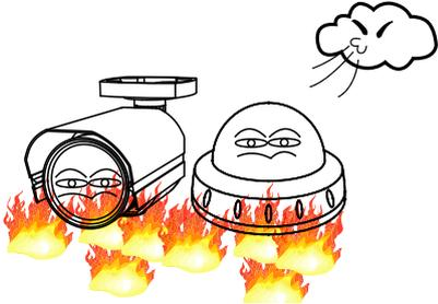
Only use the camera under conditions where temperatures are between  $-10^{\circ}\text{C}$  and  $+50^{\circ}\text{C}$ . Be especially careful to provide ventilation when operating under high temperatures.
