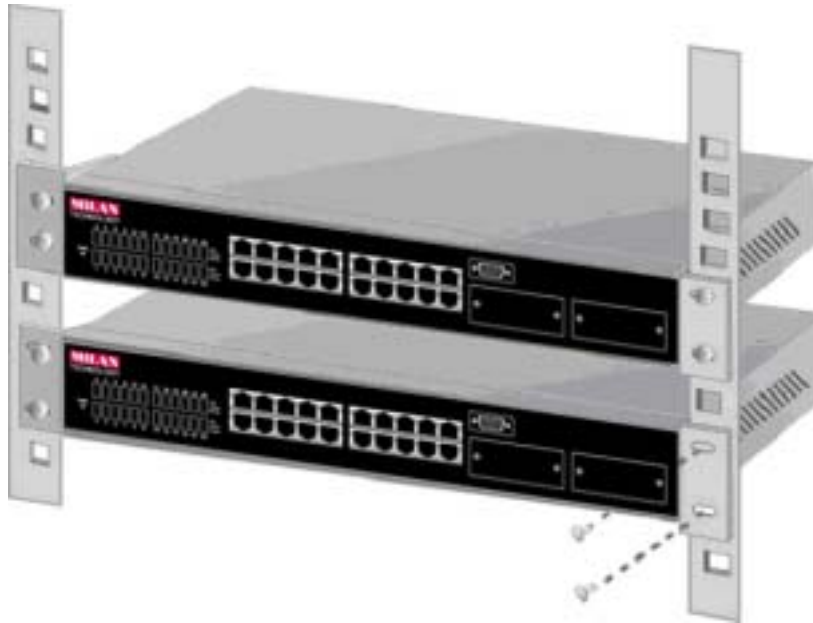
Figure 3-3. Mount the MIL-S3580 in an EIA Standard 19-inch Rack
