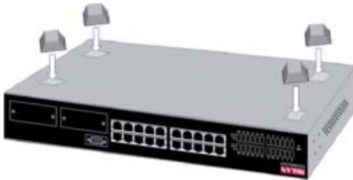
Figure 3-1. Attaching rubber feet on the bottom of the switch
