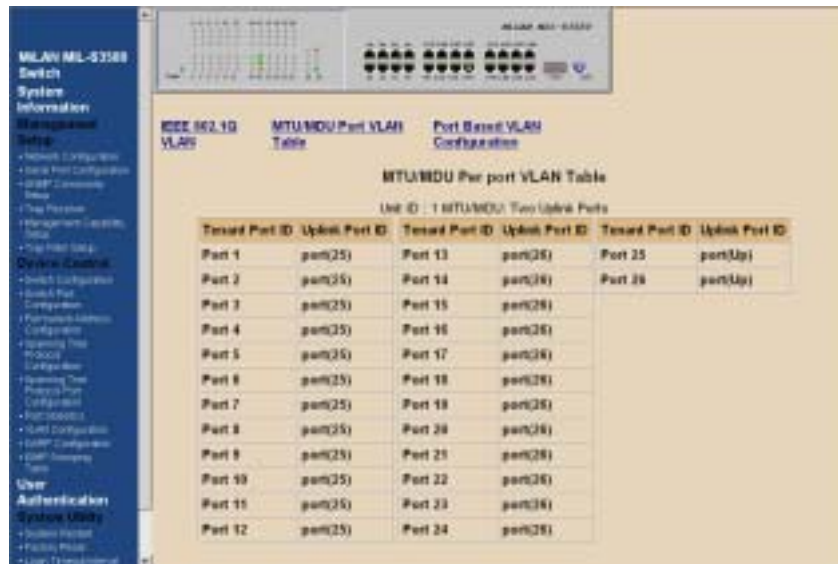
Figure 4-24. MTU/MDU Per Port VLAN Table in The VLAN Configuration Menu
