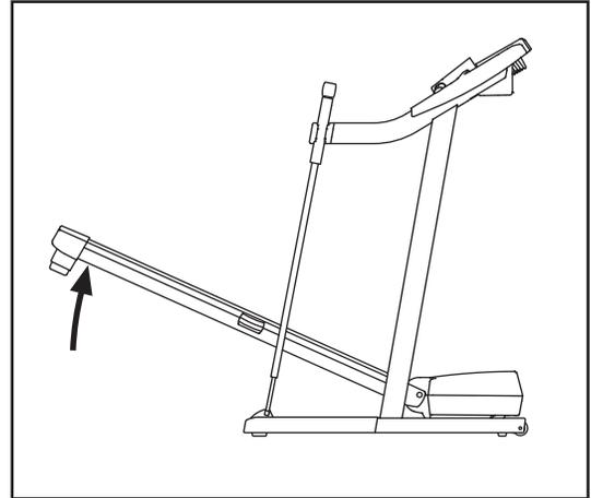
2. Move your right hand to the position shown and hold the treadmill firmly. Using your left thumb, press the storage latch to the left. Raise the treadmill until the storage latch closes over the catch. **Make sure that the storage latch is fully engaged over the catch.**
