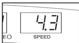
Note: The console can display speed and distance in either miles or kilometers. To see which unit of measurement is selected, hold down the Stop button, insert the key into the console, and continue to hold the Stop button for a few seconds. An “E” for English miles or an “M” for metric kilometers will appear in the display. Press the Speed + button to change the unit of measurement. When the desired unit of measurement is selected, remove the key and then reinsert it.
