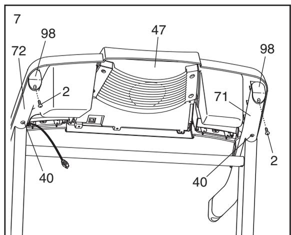
8. **Touch the Right Handrail (72) to discharge any static.** Insert the end of the Upright Wire (42) into the socket in the bottom of the Console Base (47). **The connector should slide easily into the socket and snap into place.** If the connector does not slide easily and snap into place, turn the connector and then insert it.
