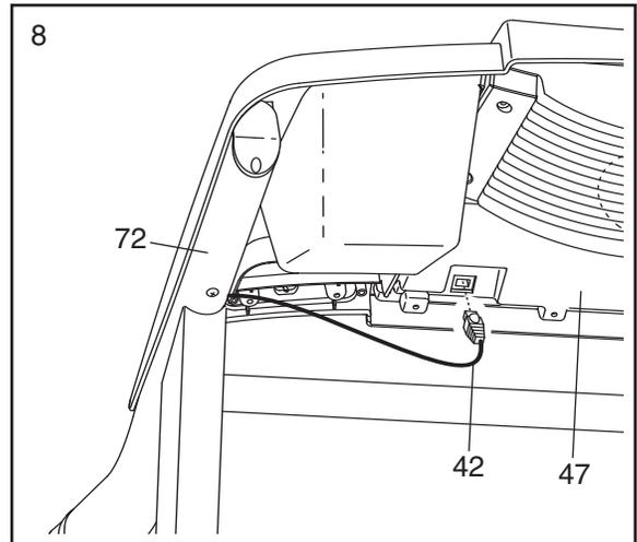
9. Press the Upright Wire (42) into the slot in the underside of the Console Base (47) in the indicated area. Cover the Upright Wire with the Right Grip Plate (36). **Be careful not to pinch the Upright Wire.** Tighten three 1/2" Screws (48) into the Right Grip Plate and the Console Base.
