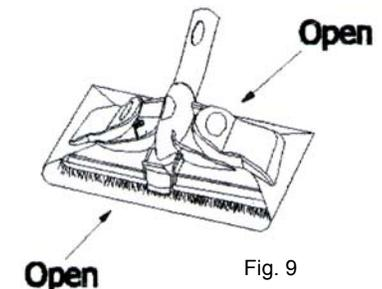
6. Place the towel around the brush, and repeat folding the towel as shown in Fig. 9. When folding the towel, leave some slack. **Do not** pull tightly around the brush, leave some looseness.
