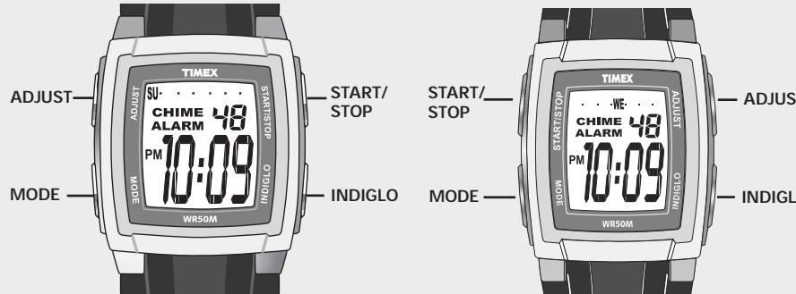
Press **MODE** to set time, date and alarm or enter Chrono Mode. Press **INDIGLO** to illuminate watch face. In any mode, press **MODE** to stop alarm beeps.
