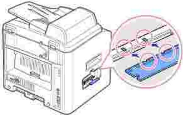
6. Insert the ends of the memory DIMM into the slot on the levers.
