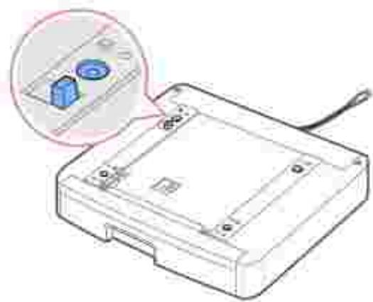
4. Place the multi-function printer over the tray, aligning the feet on the multi-function printer with the positioners in the optional Tray2.
