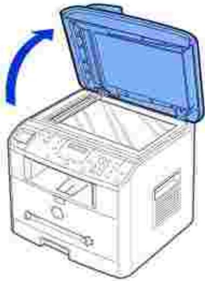
2. Place the document *face down* on the scanner glass and align it with the registration guide on the top left corner of the glass.
