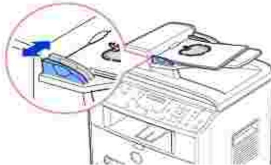
2. Make sure that the bottom of the document stack matches the paper size marked on the document input tray.
