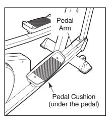
ions to the desired positions. Make sure that both pedal cushions are in the same position.
