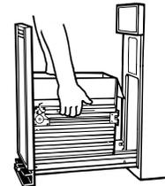
4. Vacuum the inside of the cabinet. Liquid spills or wet trash should be cleaned up by hand, or by using a vacuum designed to pick up liquids.
