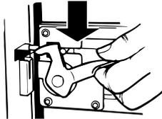
4. Lift bag by bag caddy handles. Remove trash bag from compactor and dispose properly.
