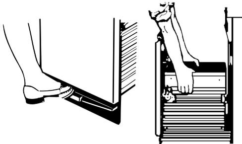
4. Place the other 2 corner posts on the floor to the side of the compactor. Grasp the sides of the compactor cabinet and put compactor on its side on top of the corner posts. Remove the shipping base from the bottom of the compactor.
