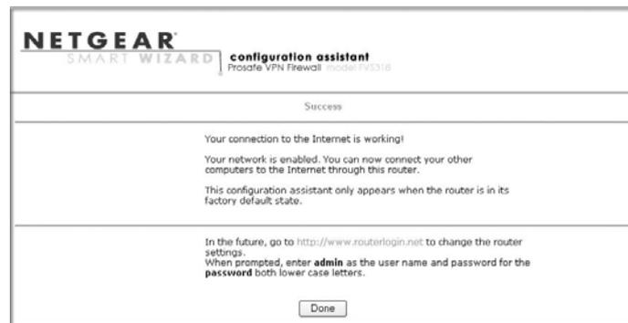
**Note:** The configuration assistant only appears when the FVS318v3 is in its factory default state. After you configure the FVS318v3, it will not appear again. You can always connect to the router configuration menu to change its settings. To do so, open a browser and go to <http://www.routerlogin.net>. Then, when prompted, enter **admin** as the user name and **password** for the password both in lower case letters.
