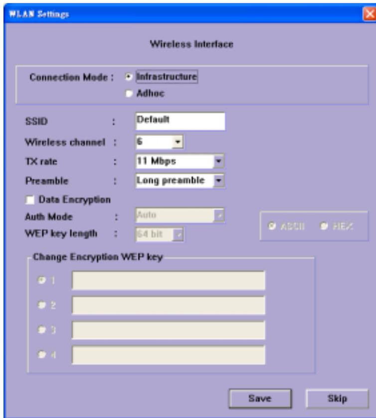
Enter the wireless LAN settings according to the access point in infrastructure or Ad Hoc master. The connection mode, SSID, WEP settings are required. If the settings are not sure at this stage, click "Skip" to continue installation in Ethernet. All the settings can be entered later from the web configuration page.
