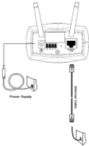
All necessary accessories can be found in the product package except for the Ethernet cable that depends on the user's environment. The Ethernet cable should meet UTP category 5 that cannot exceed 100 meters.
