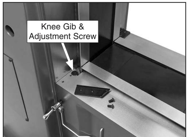
**Figure 64.** Knee gib and adjustment screw.
