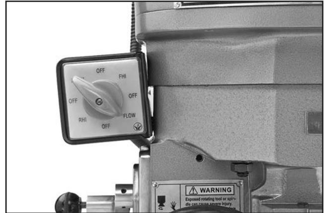
**Figure 14.** Model G0747 spindle switch.
