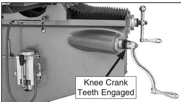
**Figure 11.** Knee crank teeth engaged.
