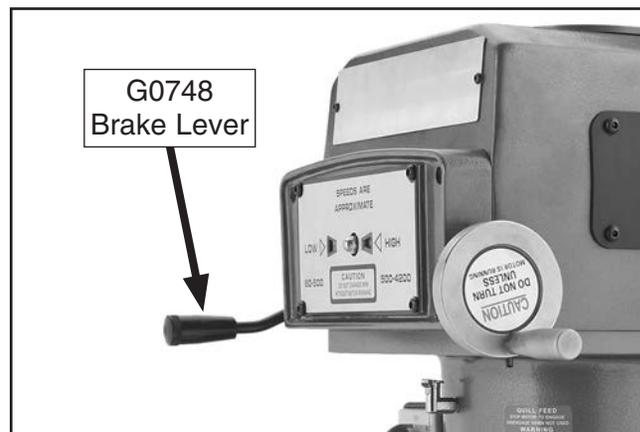
**Figure 40.** Model G0748 brake lever.
