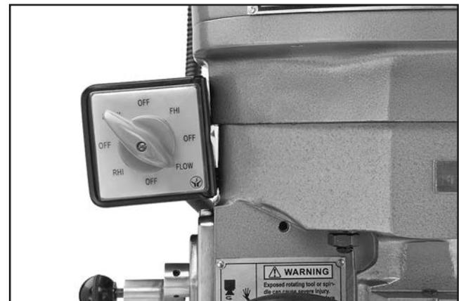
**Figure 31.** Model G0747 spindle switch.
