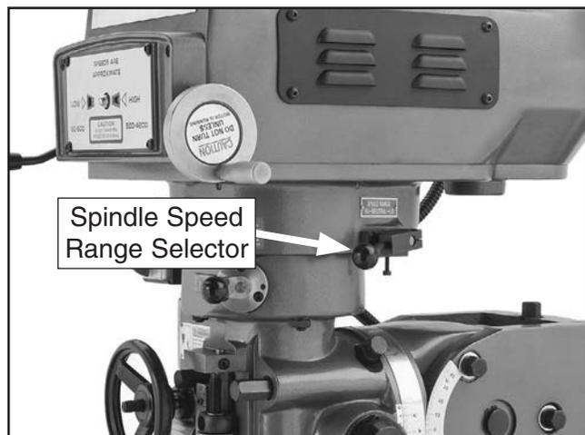
**Figure 32.** Model G0748 spindle speed selector.
