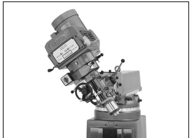
Figure 21. Head rotated to the left.
