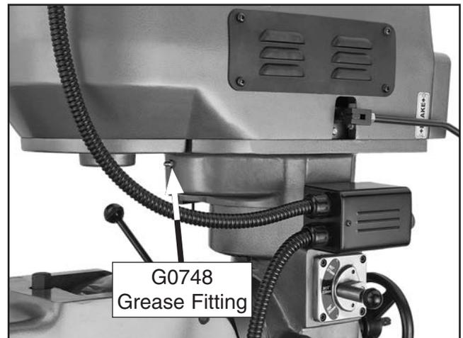
**Figure 55.** Model G0748 headstock gearing grease fitting.
