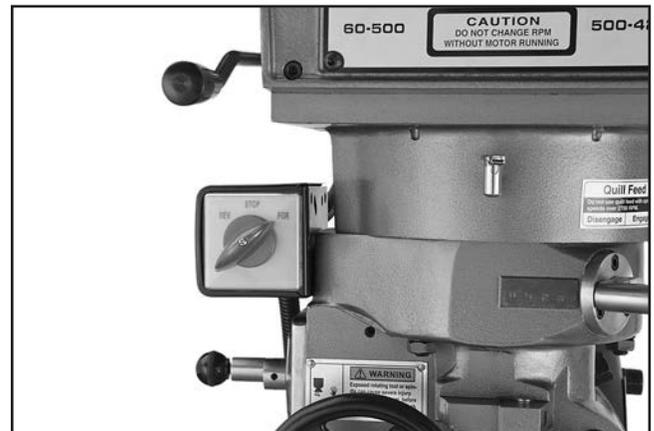
**Figure 15.** Model G0748 spindle switch.
