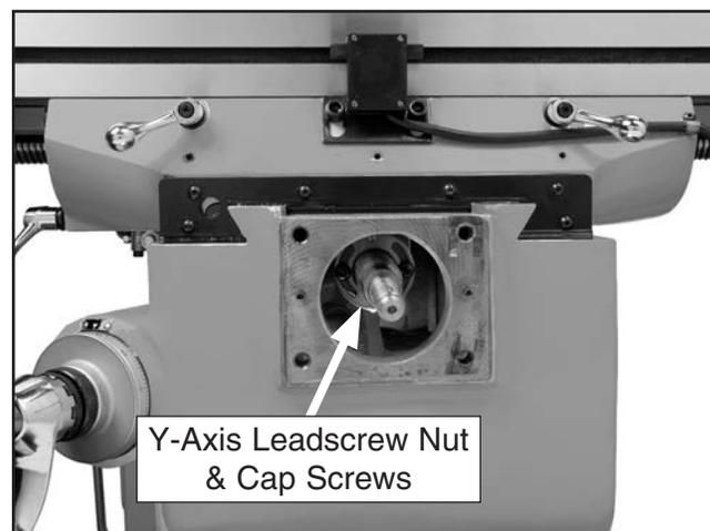
**Figure 68.** Y-axis leadscrew nut and cap screws.
