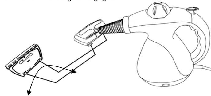
To remove the window squeegee from the steam diffuser, just push your thumb against the locking tab on the window squeegee.
