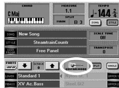
The UPPER1 field below "GUITAR MODE" shows the name of the currently selected guitar sound. You cannot select other guitar sound for UPPER 1 simply by pressing this field: press the "GUITAR MODE" field to jump to the page shown above, then change the settings you don't like. (UPPER2's guitar sound is assigned automatically and can never be changed.)
