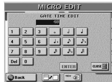
Here, you can either set the required length as a CPT value (♩ = 120CPT) or use the note icons to avoid lengthy calculations. The maximum duration a note event can have is 65,535 clocks.
