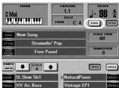
The "main page" is the E-60/E-50's display page that provides a maximum of relevant information and allows you to select (and change) items you may need during normal operation.
