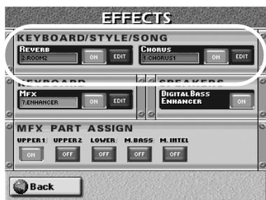
On this page, you can switch the CHORUS processor on and off by pressing the **[OFF/ON]** button icon to the right of its "display".
