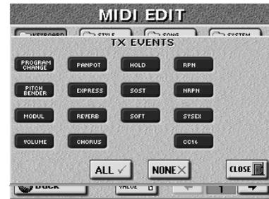
Press the ALL field to switch all button icons on (the corresponding messages are then transmitted). Press NONE to switch all button icons off. Press CLOSE to return to the page where you came from. You can also switch the following button icons on/off individually:
