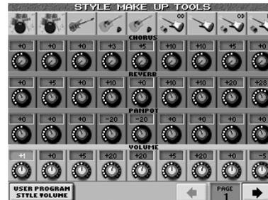
(The difference between these two pages is that the “USER PROGRAM...” settings can be saved to a User Program, and are therefore “temporary” modifications of the Style data, while the “STYLE MAKEUP TOOLS” settings can be “burned” into the Style itself.)
