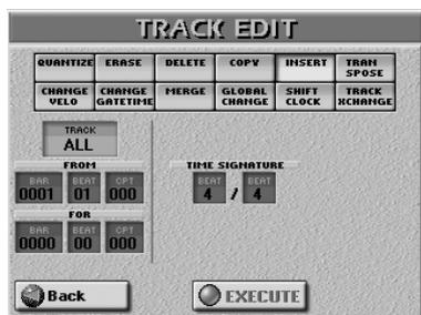
INSERT allows you to insert space and shift data that lie behind the FROM position further towards the end of the song (this is the exact opposite of DELETE). These empty measures can be "filled" using the COPY function or by recording new phrases in that area (using PUNCH IN/OUT, for example). (page 133).
