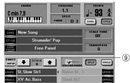
Pressing the ⑨ field takes you to the GUITAR MODE page. Note that this field can either contain an electric guitar or an acoustic one to indicate the kind of instrument you selected.
