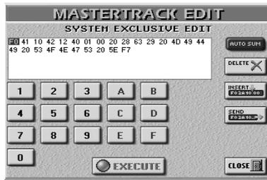
Use the **[◀▶]** buttons to select a byte (a pair of numbers) in the current line and **[▲▼]** to change lines.
