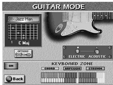
The **[Off/On]** switch icon allows you switch the Guitar mode on or off. If you selected this page by pressing EASY SETTING **[GUITAR]**, it is already set to on.
