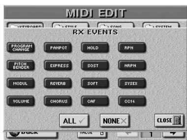
The RX events are the same as the TX events, except for the "CAF" parameter (reception of Channel After-touch messages), which can be received – or filtered.
