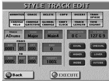
The CHANGE VELO function allows you to modify the dynamics (called "velocity") of a track or excerpt. See p. 135 for details. Only note events can be changed.
