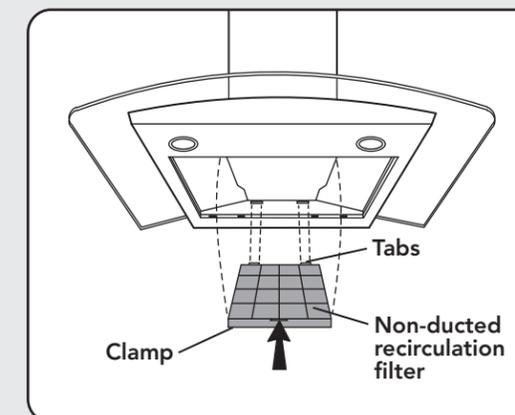
The non-ducted recirculation filter should be changed whenever the central segment of the display starts blinking (i.e. every 120 hours of operation). To remove the filter, press inward on the clamp and rotate the filter downward until the two tabs can be removed from the housing.
