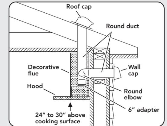
1. Decide where the ductwork will run between the hood and the outside.
