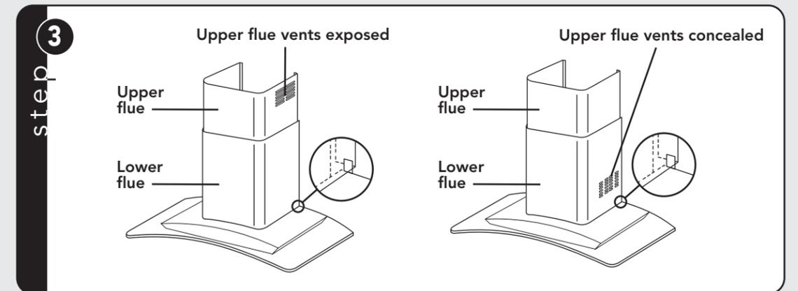
Carefully place the lower decorative flue into the recessed area of the range hood top. Carefully slide the upper decorative flue down inside the lower flue.
