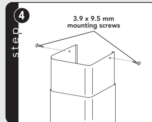
Raise the upper flue until its holes align with holes in the flue mounting bracket (located on ceiling). Secure the flue with two mounting screws.
