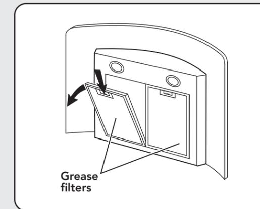
The grease filters must be cleaned approximately once every 30 hours of operation (when the central segment on the display goes on or starts blinking). Use a warm detergent solution. Grease filters are dishwasher safe. Remove filter by pushing filter towards the back of hood and rotating filter downward.
