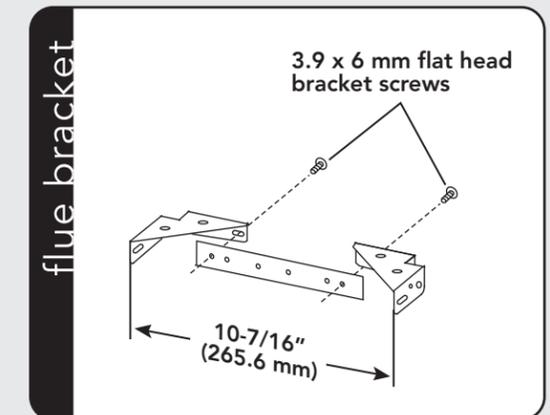
1. Assemble the flue mounting bracket, adjusting outside width as shown.
