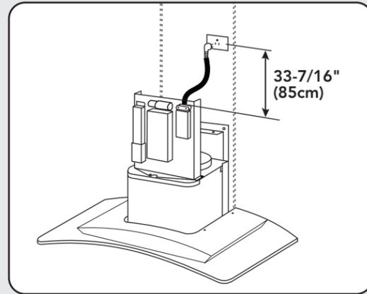
This appliance must be grounded. In the event of an electrical short circuit, grounding reduces the risk of electric shock by providing an escape wire for the electric current. This appliance is equipped with a cord having a grounding wire with a grounding plug. The plug must be plugged into an outlet that is properly installed and grounded.
