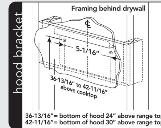
1. Construct wood wall framing that is flush with interior surface of wall studs. Make sure:
