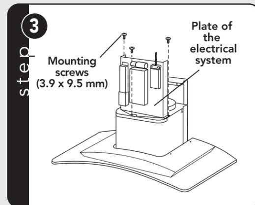
Mount the plate of the electrical system attaching it with three mounting screws (3.9 x 9.5 mm).
