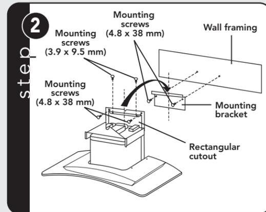
Align the rectangular opening on the back of the hood with the wall-mounting bracket. Gently lower the hood until it securely engages the bracket. Level the hood with two mounting screws (3.9 x 9.5 mm) and secure with two mounting screws (4.8 x 38 mm). Use drywall anchors provided if wall studs or framing are not available.
