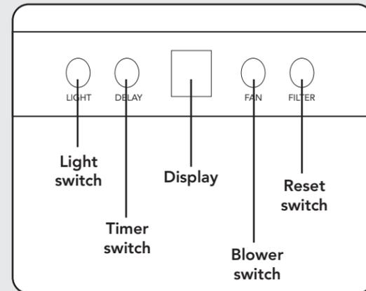
The hood is operated using the four push-buttons located at eye-level, on the front edge of the hood.
