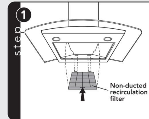
Purchase a non-ducted recirculation filter from your dealer. Install the filter by pressing the two tabs on the filter down into the special housing and rotating upward.
