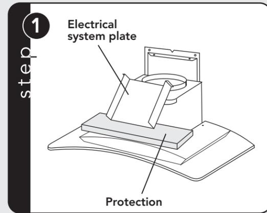
Remove the tape on the electrical system plate; place the electrical system plate on the hood (use a protection).
