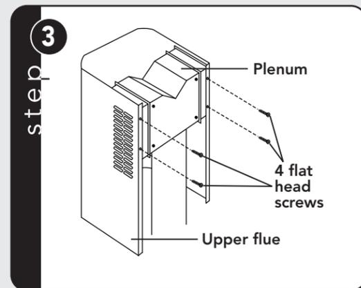
Secure the recirculation plenum to the upper flue with four flat head screws.
