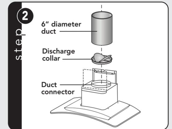
Install the discharge collar into the duct connector of the range hood. Attach an adequate length of 6" round steel ducting to the range hood duct connector.
