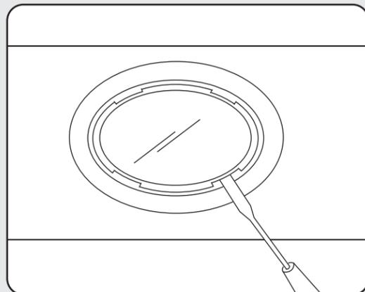
This range hood requires two halogen bulbs (max 20W, 12V, Type T3 bulb, G4 Base).
