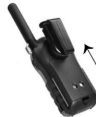
2. Locate the clip on the battery cover. Use your fingernail to gently prise open the battery cover and remove.
