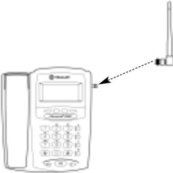
Figure 5 - Attach the antenna.
