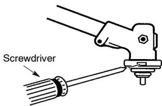
9. Tighten blade nut firmly with a wrench while holding screwdriver in position.
