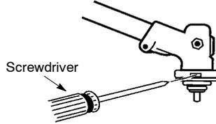
3. While holding the screwdriver in position, thread trimmer head onto the shaft by turning counterclockwise. Tighten until secure.
