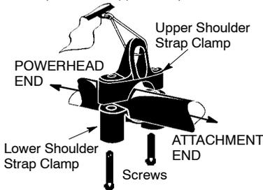
3. Insert two screws into the screw holes.
