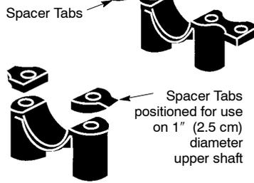
1. Place the upper shoulder strap clamp over the upper shaft above the handlebar.
