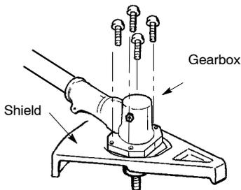
2. Insert and thread the 4 mounting screws through the holes of the gearbox and the metal shield. Tighten evenly and securely with the hex wrench provided.
