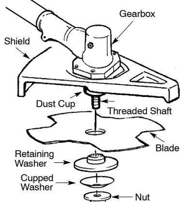
**NOTE:** Make sure all parts are in place as illustrated, and the blade is sandwiched between the dust cup and the retaining washer. There should be no space between the blade and the dust cup or the retaining washer.
