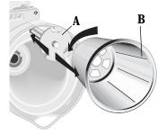
Attach shaft (A) to desired cone (B). Insert square end of shaft in square opening of housing and tighten by turning cone clockwise. Reverse to remove. Insert the cone assembly into housing (C) so shaft fits into square hub socket. As you insert the cone assembly, lift up on the latch (D) and turn the cone assembly until it fits squarely in the attachment hub.
