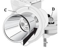
Lower the latch and pull on the cone assembly to make sure it is locked in place. To disassemble, reverse the assembly process.
