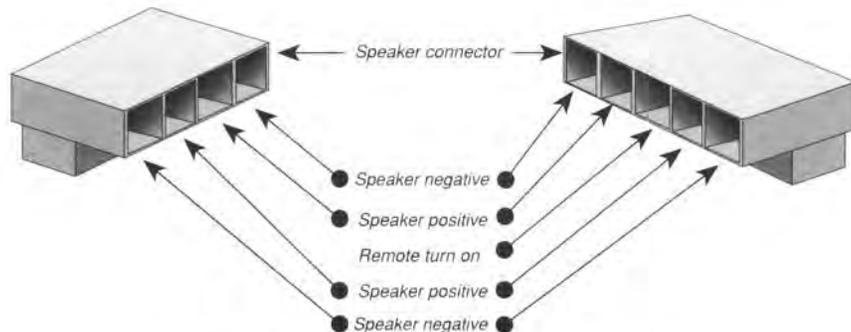
Figure D. Speaker / Remote Turn-On Connector
