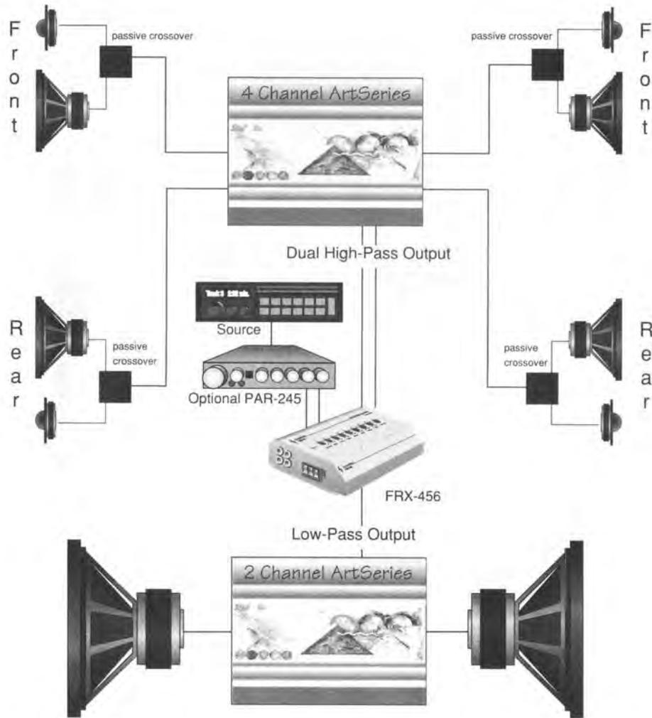
**Bi-amp System utilizing FRX-456 crossover with front/rear fade capability**
