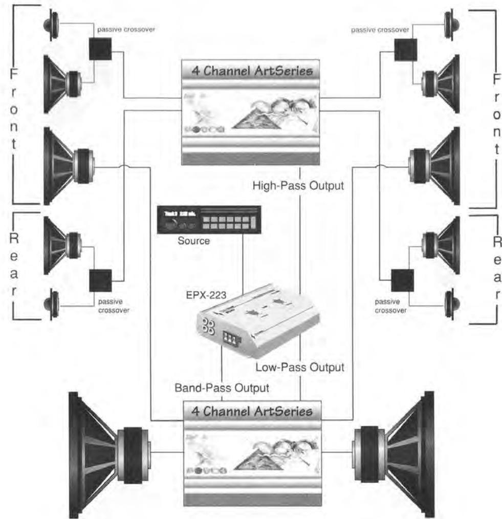
**Bi-amp System utilizing EPX-223 crossover band-pass output for front mid-bass drivers**
