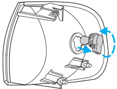
6. Insert the glass end of the new bulb into the parking lamp assembly socket. When the grooves in the plastic base are aligned, push the bulb into the socket until the plastic base contacts the rear of the socket.
