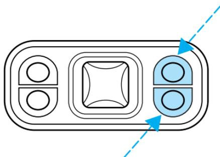
Press the control to move the seat forward, backward, up or down.
