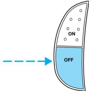
Once speed control is switched off, the previously programmed set speed will be erased.
