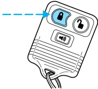
If the doors are not closed and you press the remote entry transmitter twice to confirm the doors are locked, the horn will chirp twice to warn you that the system is not arming.
