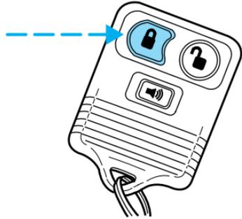
If a door is open, the system is prearmed and is waiting for the door to close. The theft indicator in the instrument panel will be lit continuously when the system is prearmed.
