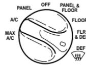
The air conditioning compressor will operate in all modes except PANEL and FLOOR. However, the air conditioning will only function if the outside temperature is about 10°C (50°F) or above.
