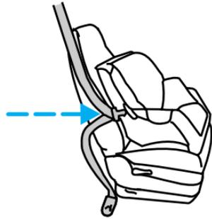
4. Insert the belt tongue into the proper buckle for that seating position until you hear and feel the latch engage. Make sure the tongue is latched securely by pulling on it.
