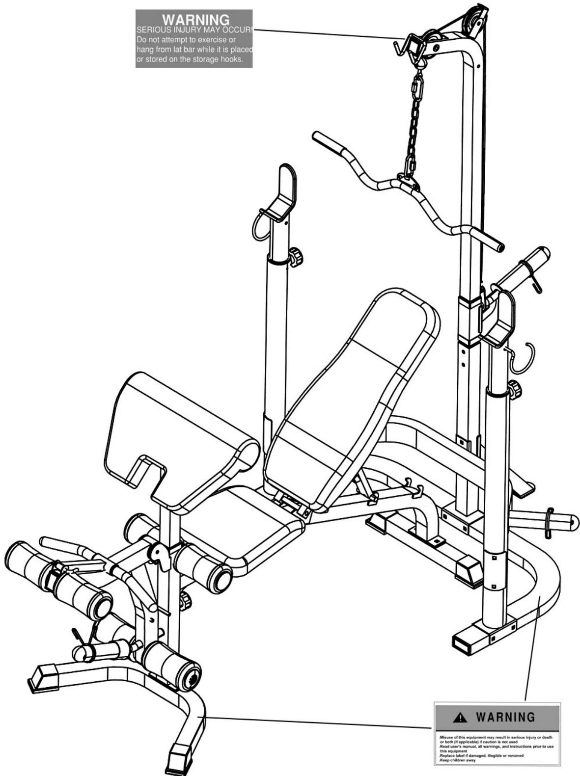
The warning labels shown here have been placed on the Front Stabilizer and Lat Bar Frame. If the labels are missing or illegible, please call customer service at 1-800-888-8899 for replacements. Apply the labels in location shown.
