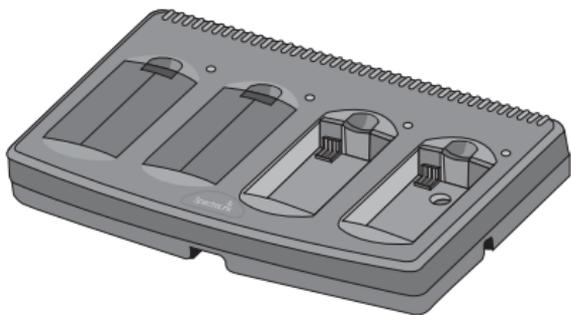
The Quad Charger is designed to simultaneously charge four Battery Packs. It may be mounted on a horizontal or vertical surface. The Battery Pack snaps into the charging slot. The LED above the occupied bay indicates the charging status of the Battery Pack in the bay.
