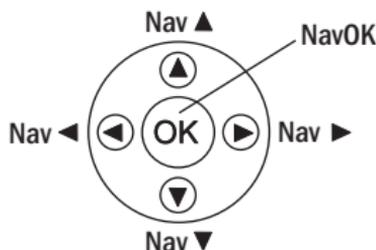
The navigation keys (Nav keys) just below the softkeys are used to navigate through menu options. These are referred to in this guide as **Nav▲**, **Nav▼**, **Nav◀**, **Nav▶**, and **NavOK**.
