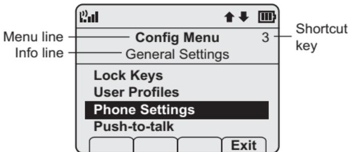
Scroll through menu options by using **Nav▲** and **Nav▼**. When an asterisk (\*) appears to the left of an option, it indicates that the option is currently selected. Press the **Exit** softkey to return to standby mode. Use the **Back** softkey to return to the previous menu.
