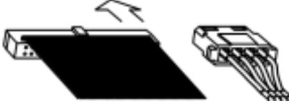
c) Attach the 4-pin power cable from the rear panel of the bottom cover to the 4-pin connector on the back of the 5.25" device.
