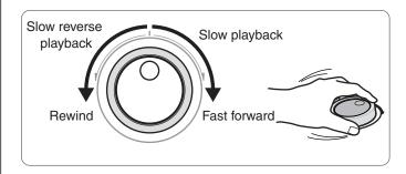
You can perform slow playback, normal-speed playback, and fast forwarding by turning this clockwise.
