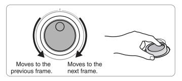
You can use this to move the position bar one frame at a time.
