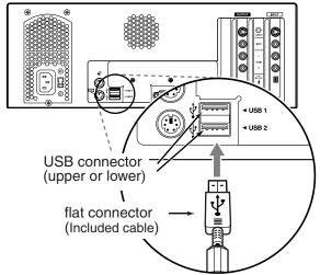
Connect with the USB connector on the front panel (Connection Example: DV-7DL)
