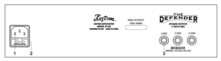
**1. AC POWER CORD RECEPTACLE:** Insert the AC cord (provided) firmly into the AC connector. NOTE: Replace the AC power cord if protective jacket is damaged or ground pin is damaged or removed. The fuse is located in a housing just below the receptacle. Replace only with same type and size. To remove the fuse, remove AC power cord and pull out on the tab above the fuse symbol located on the fuse carriage. Place the new fuse in the carriage clip and re-insert.
