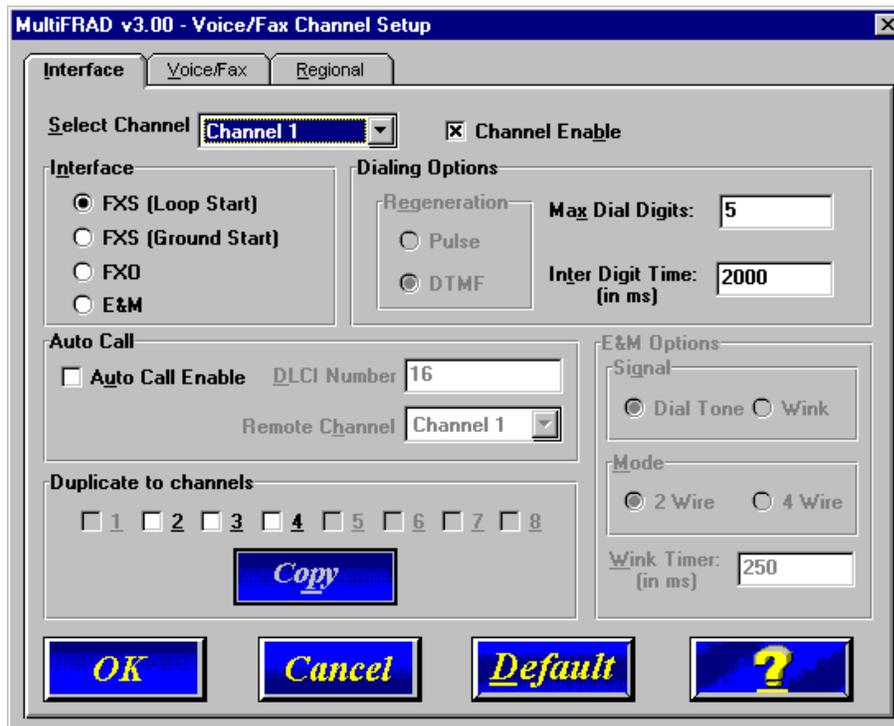
Configure each channel for the type of interface you are connecting to. The Interface tab defaults to **Channel 1** in the **Select Channel** group. To change the channel number, click the down arrow for the Select Channel and a drop-down list displays all the channels displayed. Highlight the channel number you want to configure.
