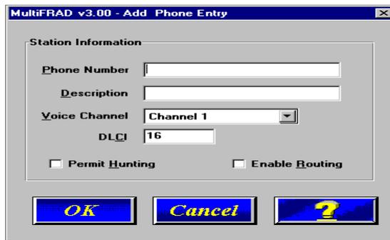
In the **Station Information** group, enter a unique phone number in the Phone Number field for one of the remote voice/fax channel you will be calling. For example, telephone number 101. This telephone number does not have to be a standard number of digits (7).
