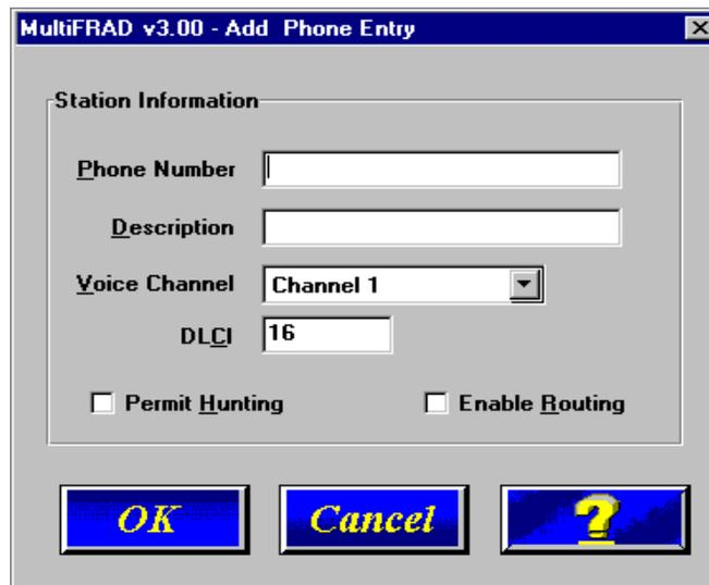
The MultiFRAD phone number does not have to be a conventional telephone number; for example, it does not have to be 717-5565. It can be a single digit or many digits with the exception that it can not be longer than the entry in the **Max Dial Digits** field in the Dialing Options group of the Channel Setup dialog box.
