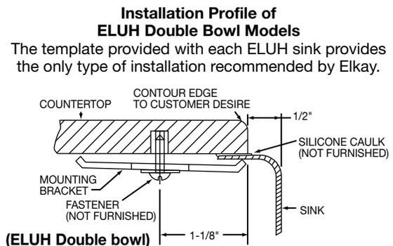
ALL DIMENSIONS IN INCHES, TO CONVERT TO MILLIMETERS MULTIPLY BY 25.4.
