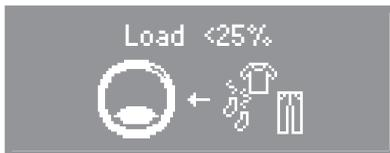
The display shows the amount of laundry loaded in the drum as a % (in 25% steps) of the maximum load permissible for the programme selected.
