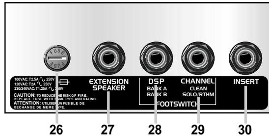
**26: FUSE:** The fuse protects the amplifier from damages caused by a faulty AC power source and/or other problems. If the fuse opens, replace it **ONLY** with the same size and type. If fuses continue to fail, check the AC source – if the source is okay, contact your Crate dealer for service information.
