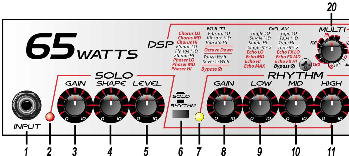
**1: INPUT:** Use this jack to connect your guitar to the amplifier by means of a shielded instrument cable.
