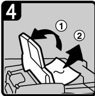
· If you cannot remove the misfed original, open the ARDF external cover, and then remove the misfed original.
