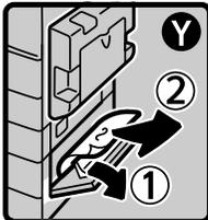
· Open the lower right cover of the optional paper tray unit and remove the misfed paper.
