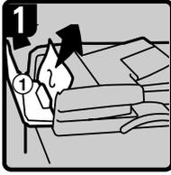
· Open the ARDF cover, and then remove the misfed original.
