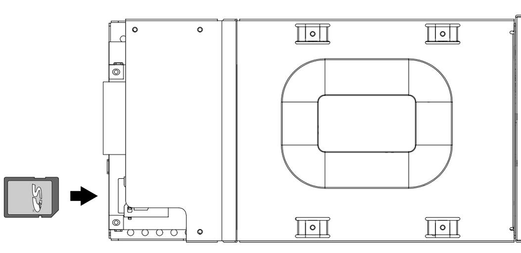
Insert the enclosed SD Memory Card firmly into the Media Player's memory card connector with the label side facing up.
