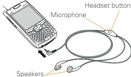
The headset button is multifunctional, and it performs different actions based on the situation. You can press the headset button to perform any of the following tasks:
