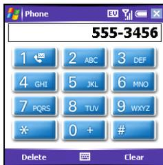
**DID YOU KNOW?** You can paste numbers directly into the Dial Pad. Copy a number from another application, switch to **Dial Pad**, and then press and hold **Center** on the **5-way** to paste the number.
