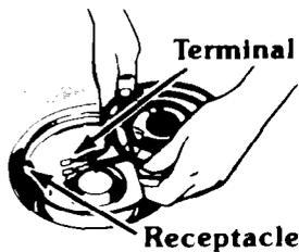
To remove surface unit, lift and pull straight out.
