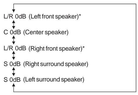
\* L or R flashes to indicate one of the front speakers from which the noise signal is output.
