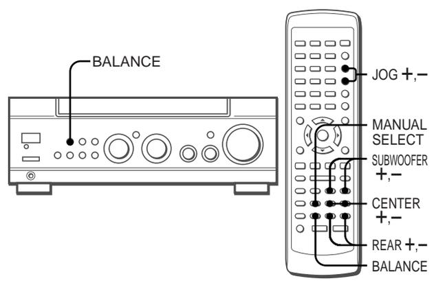
The unit is equipped with a built-in test signal generator called a noise sequencer for easy balance adjustment of all five channels. The sequencer outputs a noise signal that “travels” from channel to channel, enabling the simple adjustment of sound level to achieve the same apparent loudness, at your listening position, from each channel.
