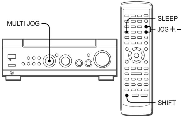
The unit can be automatically turned off at a specified time.
