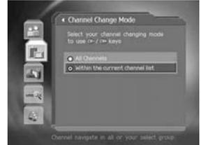
**Note:** When **Within the current channel list** in **Favourite Group** option is selected, you can only change the channel within the current channel list. To change the channel in another channel list in which the current channel list is not located, change the channel list or select **All channels** option.
