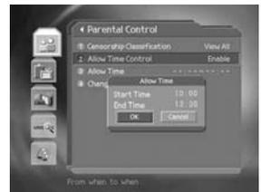
**Note:** Once the setting has been completed, you can watch programme only while the time specified by Allow Time. Or you should enter the Password to watch any programme during unspecified time.
