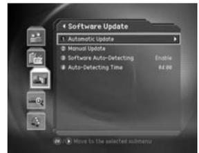
2. Automatically search for new software. Select **Stop** and press the **OK** (⊙) button to finish Search.
