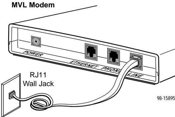
3. Connect a telephone (optional); go to Step 4 if you are not connecting a telephone to the MVL modem.
