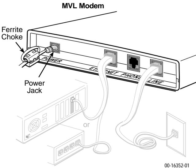
The MVL modem hardware installation is now complete. When the power cord is installed, the MVL modem goes through a power-on self-test.
