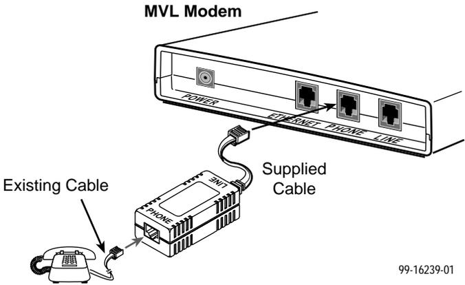
4. Use an 8-pin Ethernet cable for the Ethernet connection. Insert one end of the cable into the jack labeled ETHERNET.
