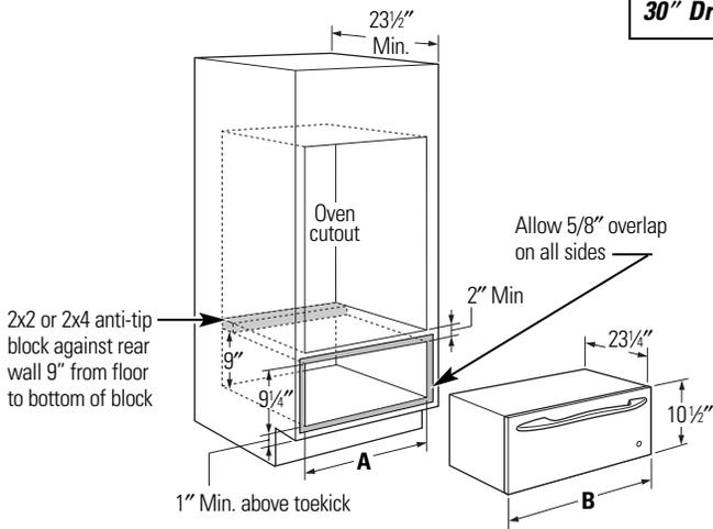
**NOTE:** Additional clearance between cutouts may be required. Check to be sure that oven supports above the warming drawer location do not obstruct the required interior 23 1/2" depth and 9 1/4" height.
