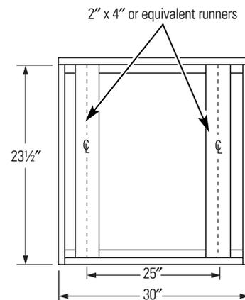
**IMPORTANT:** When installed below a single or double oven, check to be sure that any oven supports above the cutout do not obstruct the 23½" required depth of the warming drawer cutout.
