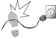
10. Protect the power cord from being walked on or pinched particularly at the plug, convenience receptacles, and the point where they exit from the apparatus.
