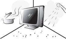
To avoid damage to power circuits, do not place the TV in locations where there is excessive steam or dust.
