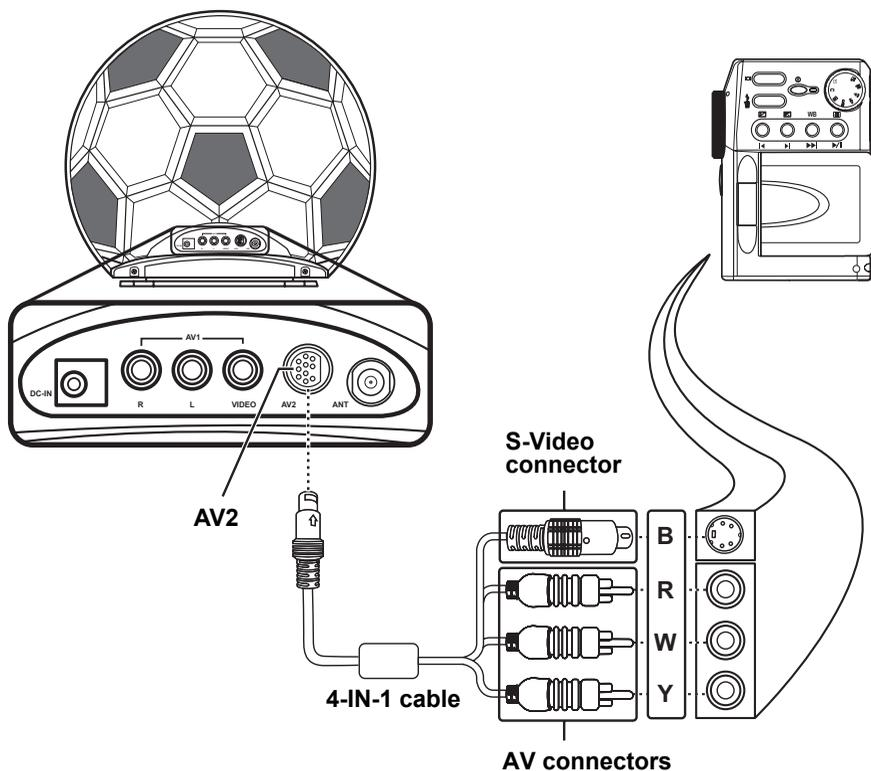
**Note:** When connecting the S-Video connector and AV connectors at the same time, the priority is given to the S-Video connector.
