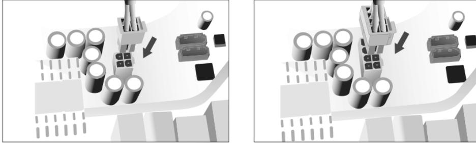
4. Connect extra cables from the cable pack to the sockets on the power supply only if needed. If you are going to plug the PCI-E cables into the PSU, they should go into the red sockets. If the red sockets are not being used for PCI-E, then they can be used for any other type of cable supplied in the pack that accompanies the PSU.
